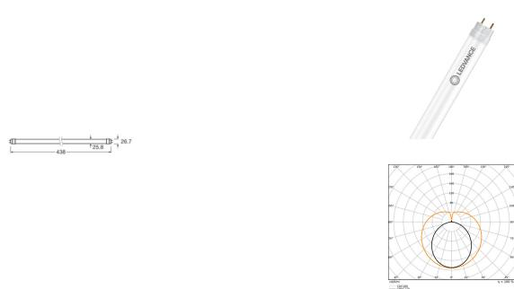
**Scheda tecnica Ledvance Tubo LED T8 EM Superior Conventional (EM), Mains (AC) Standard Output 5.1W 810lm - 830 Luce Calda - | 44cm - Sostitutiva 15W**
